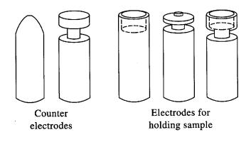
Sample pressed into electrode or mixed with Cu powder and pressed - briquetting
