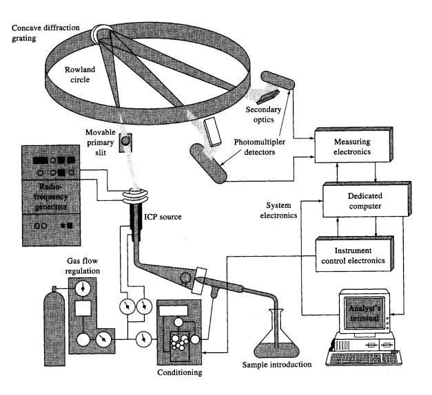
Sequential instrument - PMT moved behind aperture plate, or grating+prism moved to focus new on exit slit
